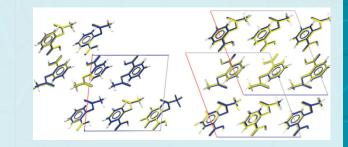
Superposition of the form-I and form-II for the predicted aspirin (PIXCRYPAR) with the experimental ones.
