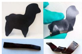
Shape memory performance of PU
