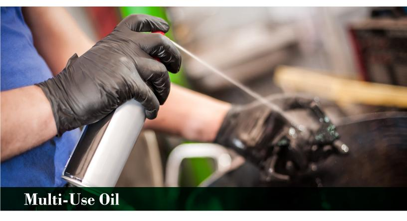
Airable has developed a soy-based oil designed to lubricate, clean, and protect metal parts. In addition to lubricating moving parts (such as hinges and gears), the oil penetrates and frees corroded components (e.g., bolts and valves) that have become stuck. It removes adhesive residue and paint and protects against rust and corrosion. In addition, this multi-use product displaces moisture to restore water-flooded equipment such as engines, spark plugs, and power tools.
