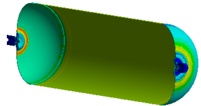
Von Mises Stresses under 500bar Pressure
