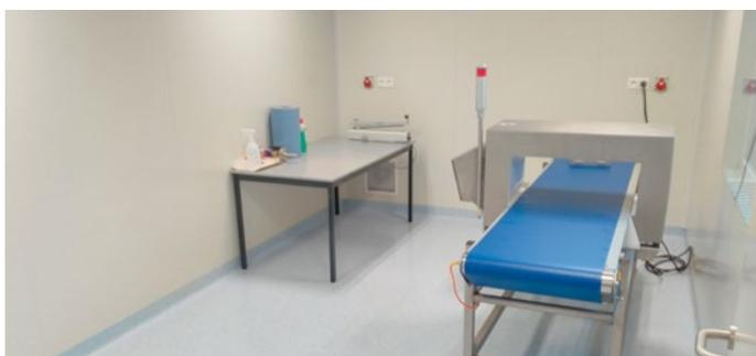
Cleanroom with a metal detector for detection of ferro, non-ferro and stainless steel contamination in packaged powders (450 mm width x 250 mm height).
