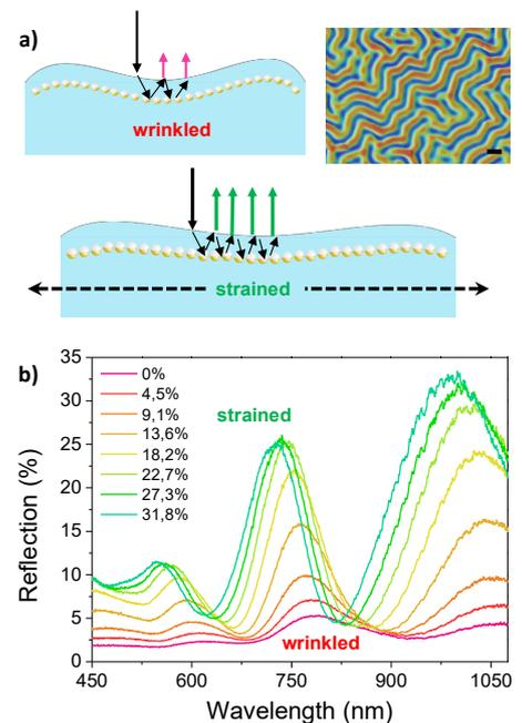
a) Schematic of the stretchable plasmonic enhanced Fabry-Perot cavity device, and b) experimental optomechanical response
