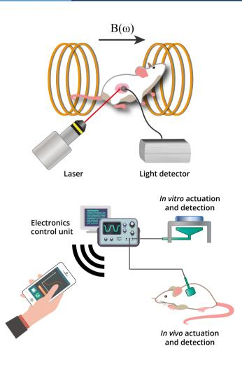
Advanced nanotherapies require sophisticated actuation and control methods. This device sees magnetic and optical heat induction mechanisms brought together in single device that allows their sequential and simultaneous application. It can find additional uses in nanothermometry for the non-invasive monitoring of local temperature variations in real time, and in the controlled release of drugs from nanostructures.
