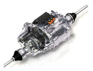
Schaeffler is also developing a two-speed electric axle (P4) for hybrid and fully electric vehicles. Marc McGrath, Schaeffler's President Automotive Americas, says that the company is targeting the system to the US small SUV and crossover market as an alternative to conventional all-wheel drive.
